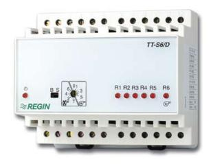
TT-S6/D is a microprocessor based step controller for controlling electric heaters etc. The step controller is controlled by a 0...10V signal from a TTC25/TTC40F regulator or from another controller or DDC.
